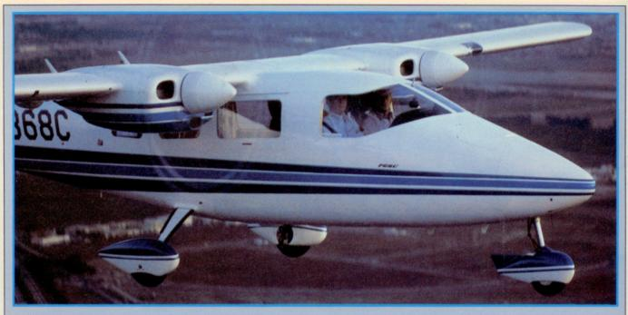
held during departure to clear a barrier, the deck angle is almost alarmingly high. Even at 100 KIAS, it is high. And remember—during departures, you do not have to worry about getting the airplane cleaned up before it will fly comfortably. The gear is fixed.
